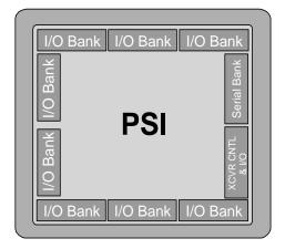
Figure 10. PSI I/O Bank Block Diagram.
