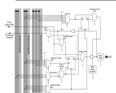
Figure 11. Block Diagram of I/O Cell.
