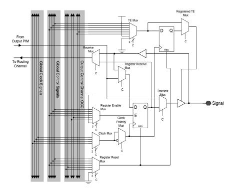
Figure 4. Block Diagram of a Standard Datapath Cell.
