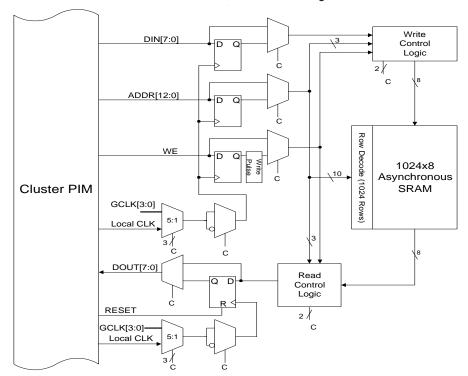
Figure 8. Block Diagram of Cluster Memory Block.
