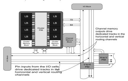
Figure 5. PSI Routing Interface.
