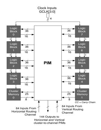
Figure 6. PSI Logic Block Cluster Diagram.
