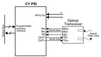
Figure 3. High-Speed PSI System Connections with an Optical Interface.
