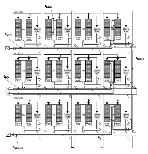
Figure 14. Timing Model for 100K gate PSI Devices.
