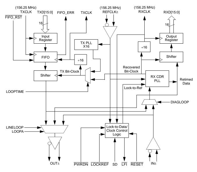
Figure 15. High Speed-PSI Transceiver Logic Block Diagram.
