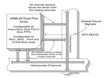
Figure 9. Block Diagram of Channel Memory Block.
